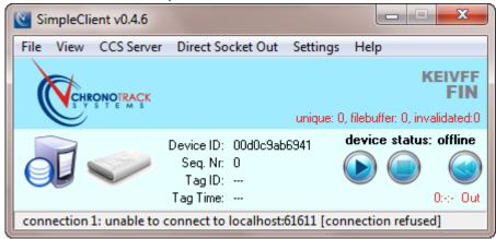
To connect to ChronoStore, use Connection 1 from the Direct Socket Out menu.
